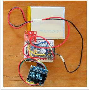
The basic ISL29125 default output is in the form of three unsigned integer values for the R, G, and B sensors. Here's some code that displays these values, adds the values for all three sensors, calculates the fraction of the total from each of the three sensors and displays the outputs on the OLED. What can these data tell us about a surface?
