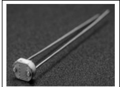
Figure 6.1. Cadmium sulfide (CdS) photoresistor.
